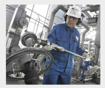
When you have to manually operate large volumes of process valves during shutdowns, Sofis EasiDrive and Power Wrench offer these operator safety and efficiency benefits:
